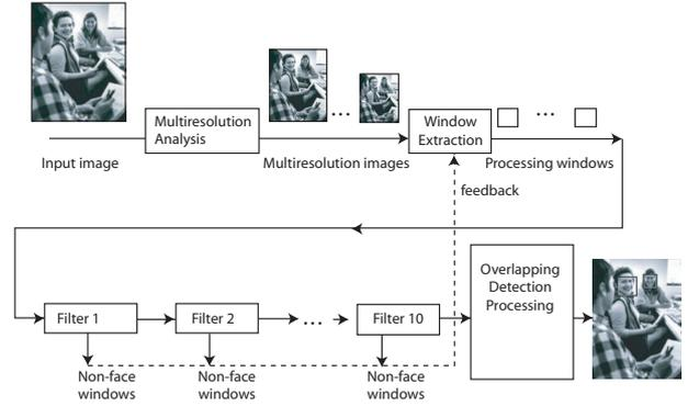
**Figure 1. Block diagram of the face detection system.**
