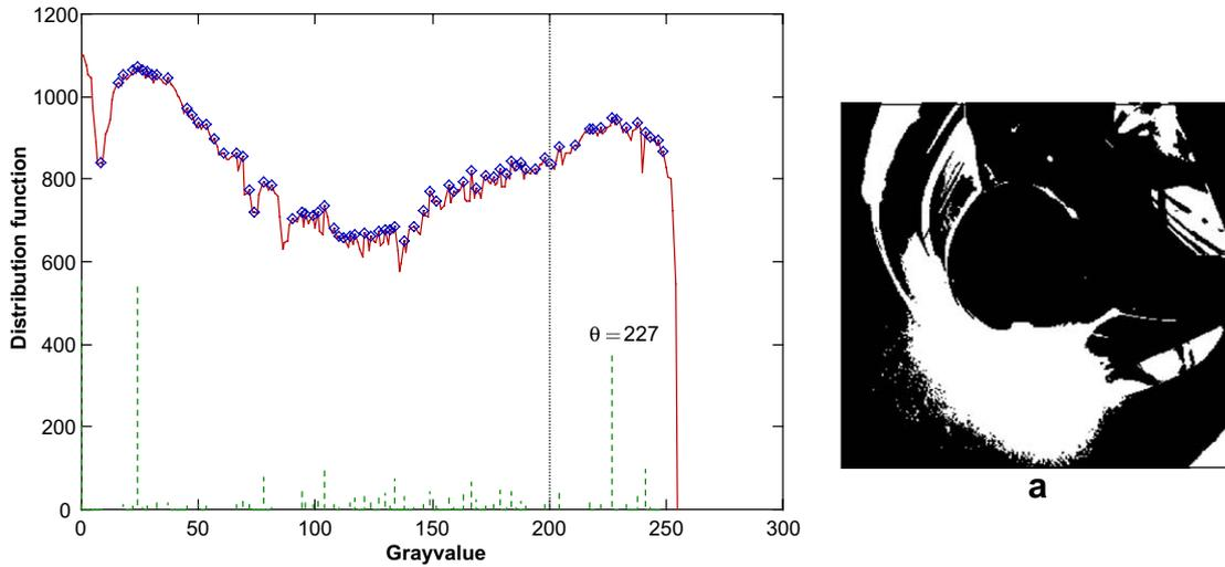
Fig. 8. Exemplary result of the computation of the peak dynamic (green dotted lines) of each local maximum (blue diamonds) on the inverted histogram (red continuous line) of the image shown in 7c. (a) Resulting binarization. (For interpretation of references in colour in this figure legend, the reader is referred to the web version of this article.)
