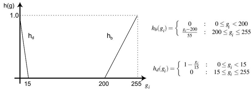
Fig. 6. Fuzzy membership functions used for image quality assessment used in the fitness function (6). The fuzzy membership function  $h_b(g_i)/h_d(g_i)$  accounts for the pixels with a low/large grayvalue  $g_i$ . The lower/larger the grayvalue, the larger the weighting in the sum.
