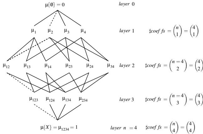
Fig. 1. Lattice structure of a fuzzy measure up to [18]. The data structure constitutes a graph with unidirectional links from  $\mu\{\emptyset\}$  to  $\mu\{X\}$ . The sorting operation of the fuzzy integral, Eq. (1), fixes up the path for the selection of the fuzzy measure coefficients. For instance a dotted line marks the path for the coefficients selected if  $x_2 > x_1 > x_3 > x_4$ , since then  $x_{(1)} = x_2$ ,  $x_{(2)} = x_1$ ,  $x_{(3)} = x_3$ , and  $x_{(4)} = x_4$ .
