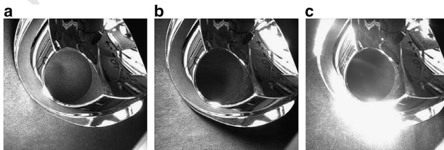
Fig. 7. Input images of the pre-processing stage of a system for the detection of structural faults on automotive headlamp reflectors (item I).
