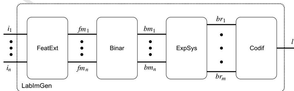
Fig. 5. Block diagram for the generation of a crisp label image in an ILFO. Signals.  $i_i$ : Input channels.  $fm_i$ : Features maps.  $bm_i$ : Binary feature maps.  $br_i$ : Binary class maps for different relationships.  $l$ : Crisp label image. Modules. *FeatExt*: Feature extraction. *Binar*: Binarization. *ExpSys*: Expert system. *Codif*: Codification.
