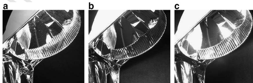
Fig. 14. Input images (of a second object) of the pre-processing stage in a system for the detection of structural faults on automotive headlamp reflectors (item II).
