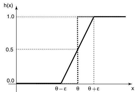
Fig. 4. Tolerance parameter  $\varepsilon$  for the fuzzification of the feature images in an ILFO with a fuzzy label image. The parameter turns the step function centered on  $\theta$  (dotted line), which would have been used as threshold for the generation of a crisp label image, into a ramp-shaped fuzzy membership function (continuous line).
